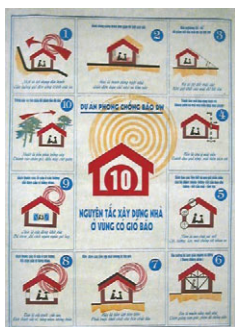
Poster : 10 key points of cyclone resistant building techniques
