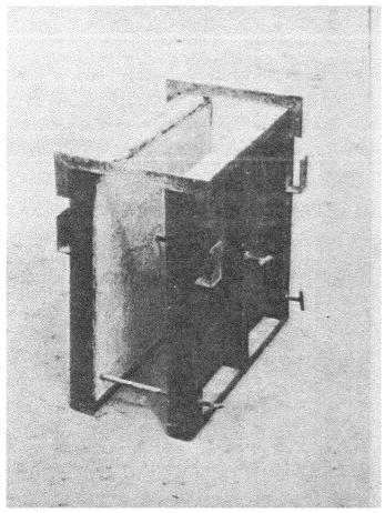
A modular straight form that put together in series connects two corners. One can see the iron bars at the bottom that are removed when the form has been tamped full.
