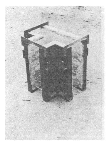
A corner form used in both centers. Notice the hooks on the top of the form holding it together.
