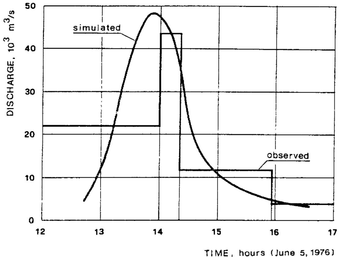
FIGURE 3 *Simulation of the outflow hydrograph due to Teton Dam Failure*
