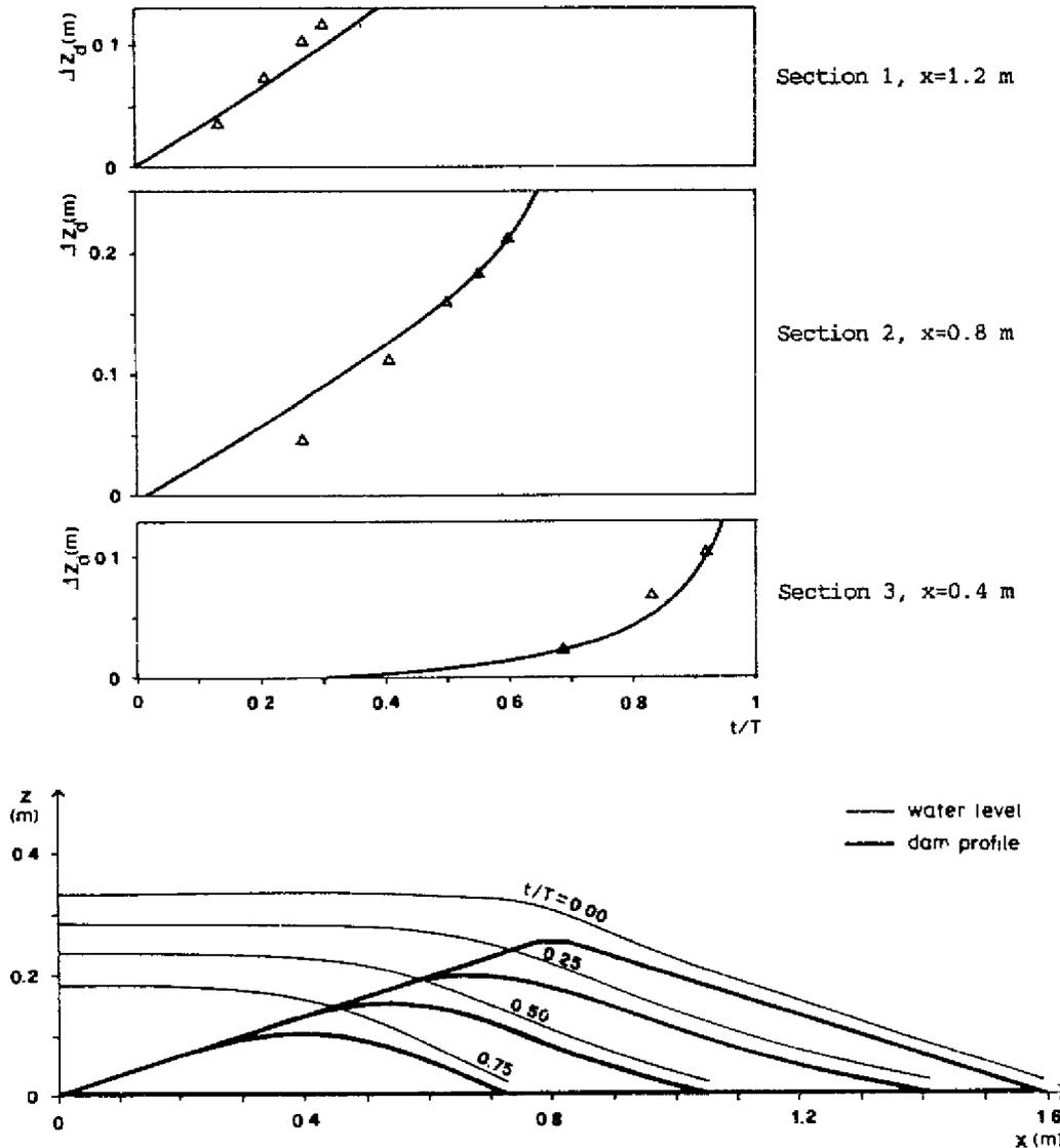
FIGURE 2 (a) – Comparison between model results and experimental data,  $T$  = complete erosion time,  $\Delta Z_d$  = sand-dyke erosion.  $\Delta$ , observed (Benoist and Nicollet, 1983), —, simulated (with Meyer-Peter and Mueller formula). Top:  $x = 1.2$  m; middle:  $x = 0.8$  m; bottom:  $x = 0.4$  m. (b) – Simulated development of water levels (fine line) and dam profiles (heavy line)
